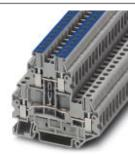
Double-level terminal block, connection method: Screw connection, cross section: 0.14 mm² - 4 mm², AWG: 26 - 12, width: 5.2 mm, color: gray, mounting type: NS 35/7,5, NS 35/15
