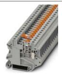
Knife disconnect terminal block, Connection type: Screw connection, Cross section: 0.14 mm² - 6 mm², AWG: 26 - 10, Nominal current: 20 A, Nominal voltage: 500 V, Length: 57.8 mm, Width: 6.2 mm, Color: red, Assembly: NS 35/7,5, NS 35/15
