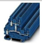
Double-level terminal block, With equipotential bonder, Connection type: Screw/plug-in connection, Cross section: 0.14 mm² - 4 mm², AWG: 26 - 12, Width: 5.2 mm, Color: blue, Mounting type: NS 35/7,5, NS 35/15
