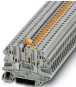
Knife disconnect terminal block, With test socket screws for insertion of test plugs, connection method: Screw connection, number of connections: 4, cross section:0.14 mm<sup>2</sup> - 6 mm<sup>2</sup>, AWG: 26 - 10, width: 6.2 mm, color: gray, mounting type: NS 35/7,5, NS 35/15
