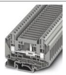
Test disconnect terminal block, connection method: Screw connection, cross section: 0.2 mm² - 10 mm², AWG: 24 - 8, width: 8.2 mm, Mounting type: NS 35/7,5, NS 35/15, NS 32, Color: gray
