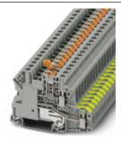
Ground modular terminal block, nom. voltage: 500 V, nominal current: 20 A, connection method: Screw connection, cross section:  $0.14 \text{ mm}^2$  -  $6 \text{ mm}^2$ , AWG: 26 - 10, length: 70.8 mm, width: 6.2 mm, color: gray, mounting: NS 35/7.5, NS 35/15, nom. voltage: 500 V
