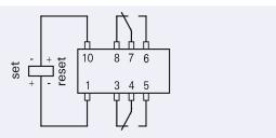
Contacts in reset position. Contact position might change during transportation and must be reset before use.
