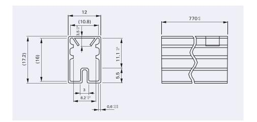
Tube for THT version 50 relays per stick 1'000 relays per box
