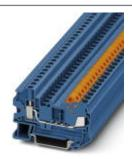
Feed-through terminal block, connection method: Quick connection, Screw connection, cross section: 0.5 mm² - 2.5 mm², AWG: 20 - 14, width: 6.2 mm, color: blue, mounting: NS 35/7,5, NS 35/15
