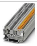
Feed-through terminal block, Connection type: Quick connection, Spring-cage connection, Cross section: 0.5 mm² - 2.5 mm², AWG :20- 14, Width: 6.2 mm, Color: gray, Mounting: NS 35/7,5, NS 35/15
