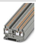
Component terminal block, with integrated 1N4007 diode, nom. voltage: 800 V, nominal current: 0.5 A, connection method: Push-in connection, number of connections: 3, cross section:0.14 mm² - 4 mm², AWG: 26 - 12, width: 5.2 mm, color: gray, mounting type: NS 35/7,5, NS 35/15
