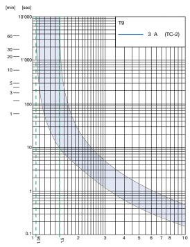
Multiple of Rated Current In Reference Temperature +23°
