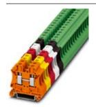
Feed-through terminal block, Connection method: Screw connection, Cross section: 0.2 mm² - 10 mm², AWG: 24 - 8, Width: 8.2 mm, Color: black, Mounting type: NS 35/7,5, NS 35/15
