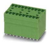
Header, Nominal current: 8 A, Rated voltage (III/2): 160 V, Number of positions: 6, Pitch: 3.81 mm, Color: green, Contact surface: Tin, Mounting: Wave soldering, In combination with MCV plug components, both an MCVW and an MCVR plug must be used.
