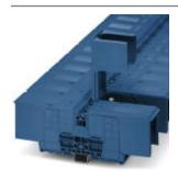
Bolt connection terminal block, Connection method: Bolt connection, Number of positions: 1, Cross section: 10 mm² - 240 mm², AWG: 8 - 500, Width: 49 mm, Color: blue, Mounting type: NS 35/7,5, NS 35/15, ct screw connection
