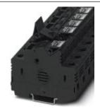
Fuse modular terminal block, Connection method: Screw connection, Cross section: 1.5 mm²- 25 mm², AWG: 16 - 4, Nominal current: 32 A, Nominal voltage: 690 V, Width: 18 mm, Fuse type: Midget / 10.3 x 38, Fuse type: Glass / ceramics / ..., Mounting type: NS 35/7,5, NS 35/15, Color: black/red
