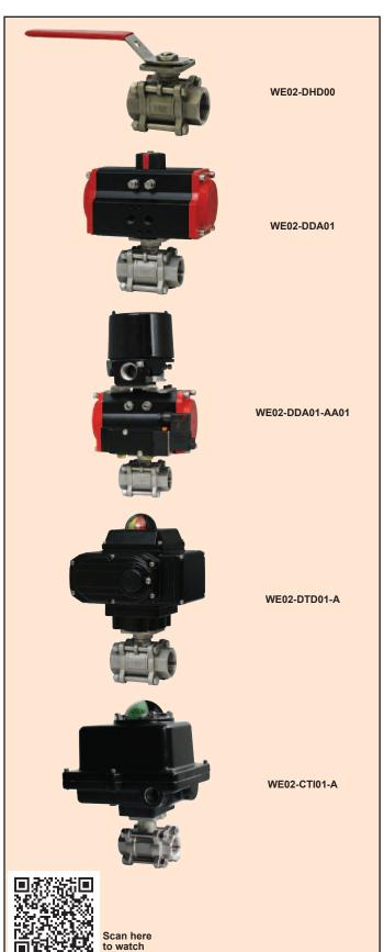
The Series WE02 incorporates a full port 3-piece SS ball valve for great flow rates with minimal pressure drop. The valve features a blowout proof stem for added safety, reinforced PTFE seats and seals for longer life, and a 316 SS (ASTM CF8M) ball for better performance. Actuators are direct mounted creating a compact assembly for tight spaces. Limit switches are able to be mounted directly to the valves allowing for remote position indication.
