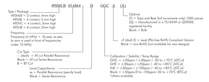
Part Number Examples: Freq 5.1234MHz,  $\pm 30$ ppm calib,  $\pm 30$ ppm stability, -20 to +70°C, 16pF = 49SMLB05.1234-16GGC
