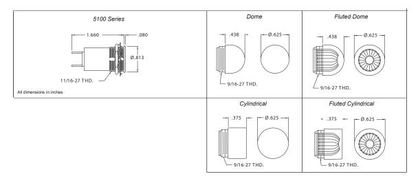
The Chicago Miniature Lamp Miniature Indicator Lights are versatile, industry standard, front panel indicators capable of accepting a variety of T-2 and T-3 1/4 miniature bayonet based incandescent and neon lamps. These indicator lights accept a variety of different lens styles an colors, and are excellent for providing a large, bright, easily noticed status indicator. The lamp is not included with this indicator light; please order the required lamp separately.
