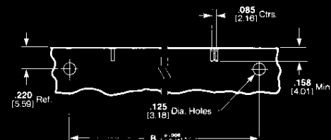
Recommended Pc Board Mounting Dimensions
