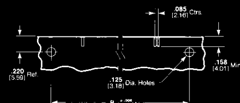
Recommended Pc Board Mounting Dimensions
