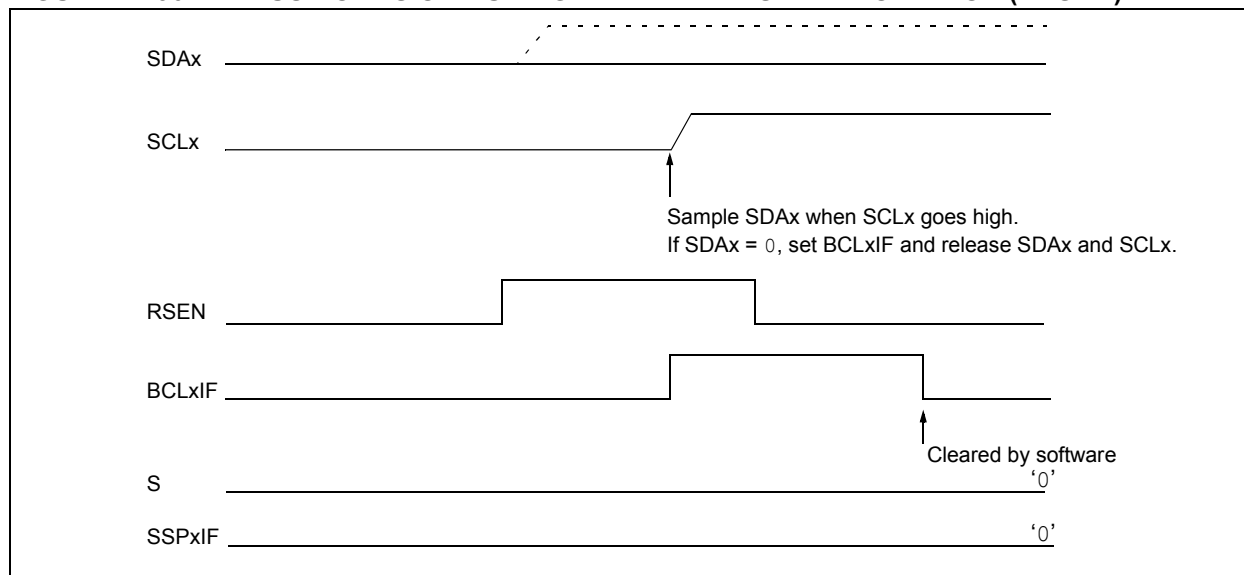
FIGURE 21-36: BUS COLLISION DURING A REPEATED START CONDITION (CASE 1)
