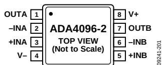
Figure 4. 8-Lead, MSOP (RM-8), ADA4096-2
