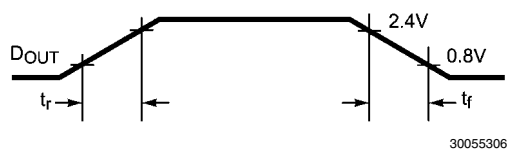
FIGURE 3. D OUT Rise and Fall Times
