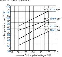
4. Ambient temperature characteristics Tested sample: AHES3191, 6 pcs.
