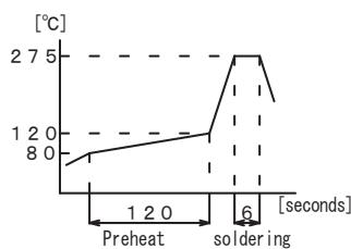
● Pre-heating should be done at temperatures ranging from 80°C to 120°C and within 120 seconds.
