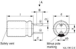
The series B41898 has no sleeve nor minus pole marking, the positive pole is marked on the aluminum case side instead.
