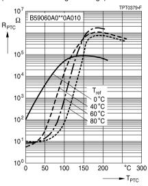
PTC resistance R<sub>PTC</sub> versus PTC temperature T<sub>PTC</sub> (measured at low signal voltage)
