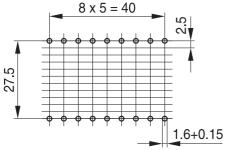
Hole arrangement View in mounting direction
