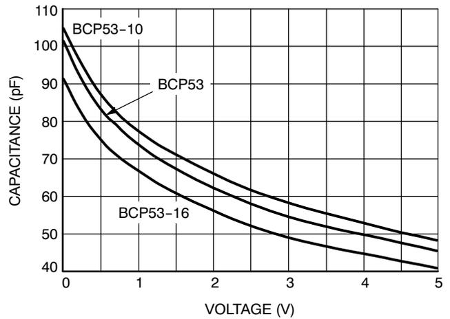
**Figure 10. Input Capacitance**
