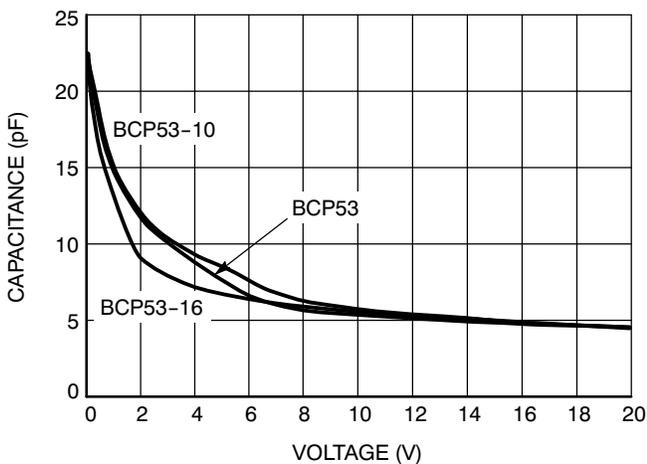
**Figure 11. Output Capacitance**
