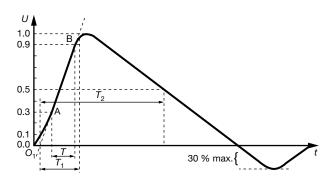
Front time:  $T_1$  = 1.67 x T = 1.2  $\mu$ s  $\pm$  30 % Time to half-value:  $T_2$  = 50  $\mu$ s  $\pm$  20 %
