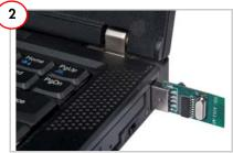
Connect the bridge dongle to the PC. The bridge enumerates as a HID device.
