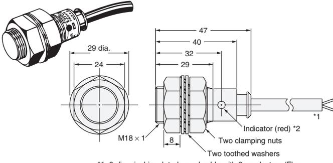
\*1. 6-dia. vinyl-insulated round cable with 2 conductors (Flame-resistant, Conductor cross section: 0.5 mm<sup>2</sup>, Insulator diameter: 1.9 mm), Standard length: 2 m
