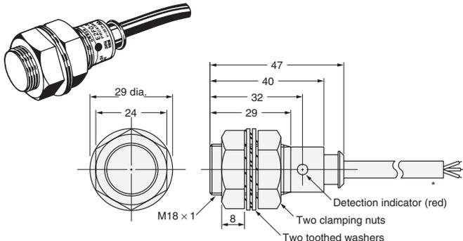
\* 6-dia. vinyl-insulated round cable with 3 conductors (Flame resistant, Conductor cross section: 0.5 mm<sup>2</sup>, Insulator diameter: 1.9 mm), Standard length: 2 m
