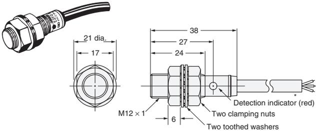
\* 6-dia. vinyl-insulated round cable with 3 conductors (Flame resistant, Conductor cross section: 0.5 mm<sup>2</sup>, Insulator diameter: 1.9 mm), Standard length: 2 m
