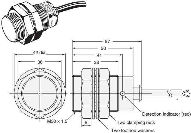
\* 6-dia. vinyl-insulated round cable with 3 conductors (Flame resistant, Conductor cross section: 0.5 mm<sup>2</sup>, Insulator diameter: 1.9 mm), Standard length: 2 m
