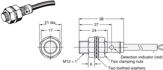
\* 6-dia. vinyl-insulated round cable with 2 conductors (Flame resistant, Conductor cross section: 0.5 mm<sup>2</sup>, Insulator diameter: 1.9 mm), Standard length: 2 m
