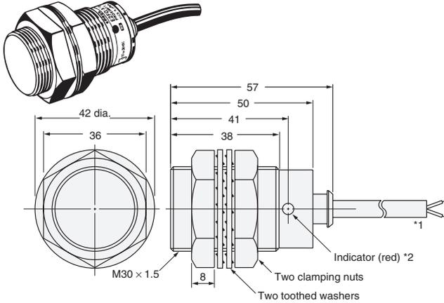
\*1. 6-dia. vinyl-insulated round cable with 2 conductors (Flame-resistant, Conductor cross section: 0.5 mm<sup>2</sup>, Insulator diameter: 1.9 mm), Standard length: 2 m
