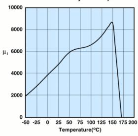
Measured on a 17/10/6mm toroid at 10kHz.
