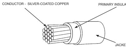
PRIMARY INSULATION - RADIATION-CROSSLINKED. MODIFIED ETFE Primary insulation shall be of a contrasting pigmentation to that of the jacket.
