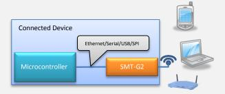
Nano WiReach SMT-G2 makes adding Internet connectivity to embedded devices a breeze. It does not require any kind of WiFi driver development on the host CPU, and its multiple interfaces (UART, SPI, RMII and USB 1.1) minimize the need to redesign the host device hardware.
