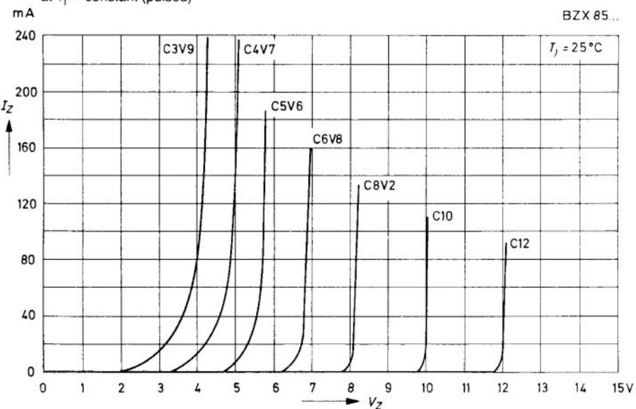
**Breakdown characteristics**at  $T_j = \text{constant}$  (pulsed)
