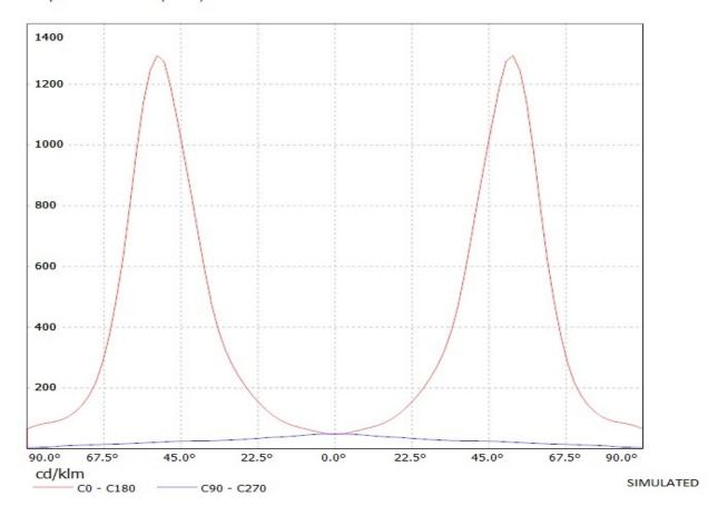
Luminaire: Ledil Oy C10757\_Strada-DW-XR C10757\_Strada-DW-XR Lamps: 1 x Cree XR-E (White)
