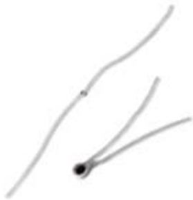
112 Series, large glass bead with adjacent leads, 10,000 Ohm resistance,  $\pm 20.0\%$  tolerance, 25/85 BETA = 3669
