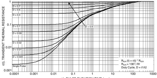
t1, PULSE DURATION TIME (sec) Figure 13 Transient Thermal Resistance
