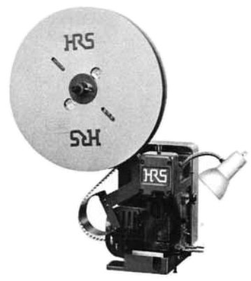
Semi-Auto Machine CM-105 (CL901-0005-4) Applicator (Die) 105-DN50 (CL901-0208-1)
