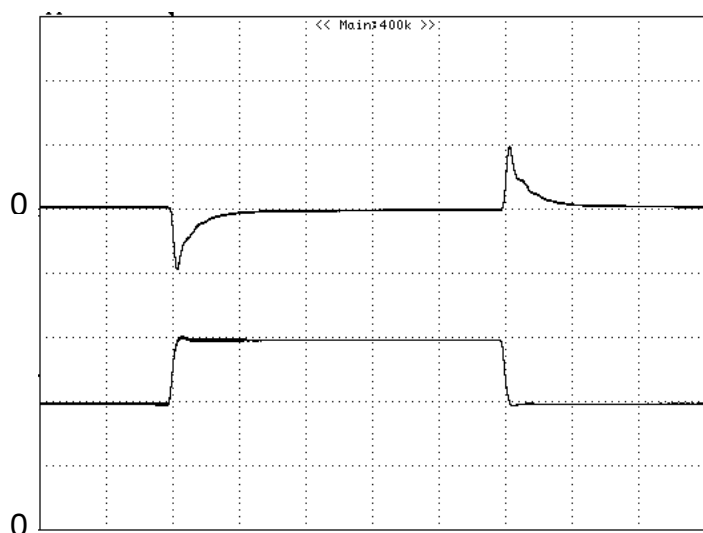
Figure 8: Output voltage response to step-change in load current (75%-50%-75% of I_o , max; di/dt = 0.1A/\mu s ). Load cap: 10\mu F tantalum capacitor and 1\mu F ceramic capacitor. Top Trace: V_{out} (0.2V/div, 200us/div), Bottom Trace: I_{out} (1A/div). Scope measurement should be made using a BNC cable (length shorter than 20 inches). Position the load between 51 mm to 76 mm (2 inches to 3 inches) from the module
