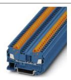
Feed-through terminal block, connection method: Quick connection, number of connections: 2, cross section:0.5 mm² - 2.5 mm², AWG: 20 - 14, width: 6.2 mm, color: blue, mounting type: NS 35/7,5, NS 35/15
