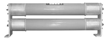
3. Back-up - defined by ANSI C37.40 as "a fuse capable of interrupting all currents from the maximum rated interrupting current down to the rated minimum interrupting current." The minimum rated interrupting current is the lowest current that the fuse will be able to clear properly. This creates a need to place a low current interrupting device in series with the back-up rated fuse.
