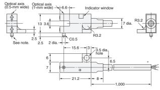
$^{\ast}$  Vinyl-insulated round cable of 3.5 dia., 3 cores, (0.14 mm² with 1.0-dia. insulator); Standard length: 1 m
