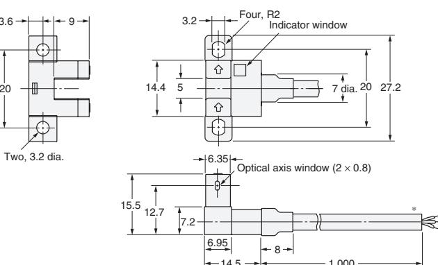
\* Vinyl-insulated round cable of 3.5 dia., 3 cores,
