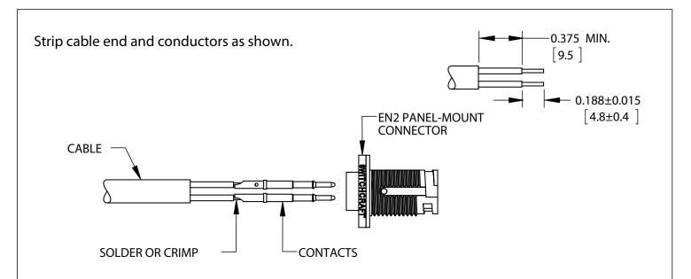
Soldering or crimping conductors to contacts is recommended before insertion into connector. If crimping, use hand or pneumatic crimp tool with crimp positioner per contact size. If soldering after contacts are inserted in the connector, limit exposure of contacts to soldering iron temperature to 4 sec. maximum. Soldering iron temperature should not exceed 650°F (343°C).
