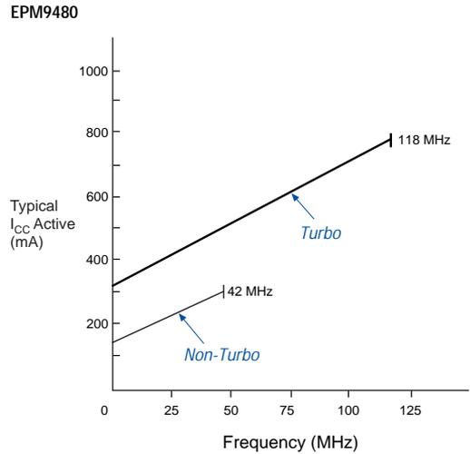
Figure 15.  $I_{CC}$  vs. Frequency for MAX 9000 Devices (Part 2 of 2)
