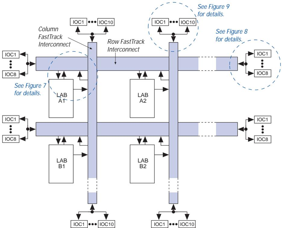
The LABs within MAX 9000 devices are arranged into a matrix of columns and rows. Table 5 shows the number of columns and rows in each MAX 9000 device.
