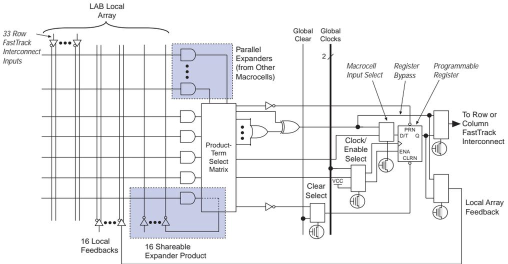
Combinatorial logic is implemented in the local array, which provides five product terms per macrocell. The product-term select matrix allocates these product terms for use as either primary logic inputs (to the OR and XOR gates) to implement combinatorial functions, or as secondary inputs to the macrocell's register clear, preset, clock, and clock enable control functions. Two kinds of expander product terms ("expanders") are available to supplement macrocell logic resources:
