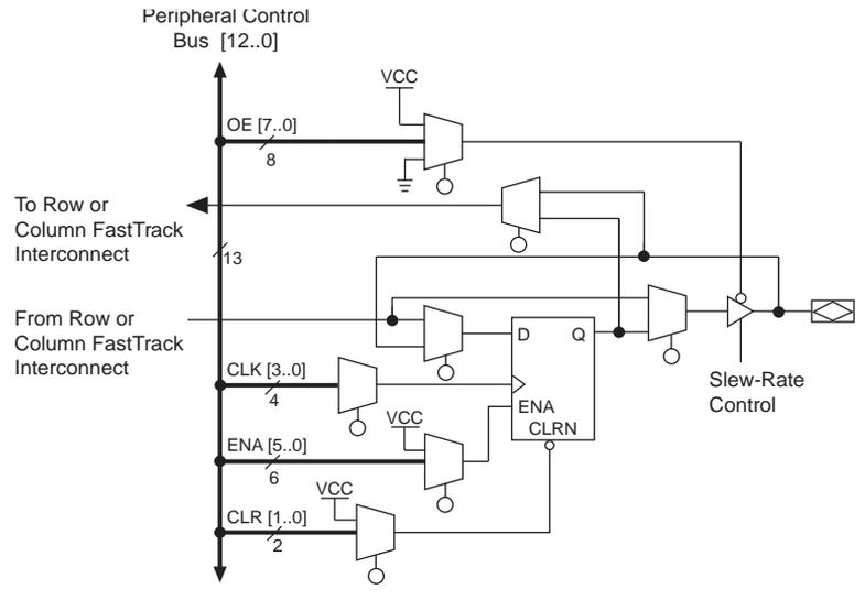
I/O pins can be used as input, output, or bidirectional pins. Each IOC has an IOC register with a clock enable input. This register can be used either as an input register for external data that requires fast setup times, or as an output register for data that requires fast clock-to-output performance. The IOC register clock enable allows the global clock to be used for fast clock-to-output performance, while maintaining the flexibility required for selective clocking.
