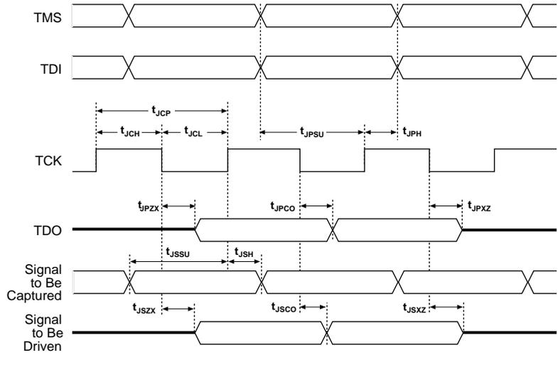
Table 13 shows the JTAG timing parameters and values for MAX 9000 devices.
