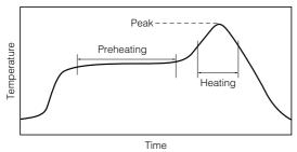
For soldering (Example: Sn/Pb)
