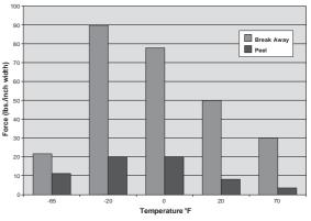
when high impact stresses along with high frequencies are encountered. At low temperatures, the tape becomes very firm and glassy; the ability to absorb impact energy is reduced.
