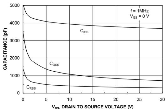
Figure 8. Capacitance Characteristics
