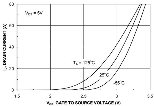
Figure 5. Transfer Characteristics
